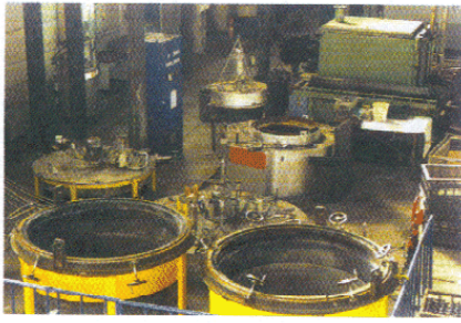
Figure 2. Process-controlled 1500 x 2000 shaft furnace complex for gas nitriding and gas nitrocarburising at Härtereie Reese Weimar
