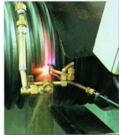
Figure 3 Flame hardening of a cable drum
